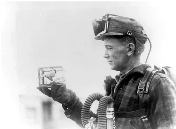
Fig. 2. A photograph (taken in 1928) of mining foreman R Thornburg holding a small cage with a canary in it. Miners used this bird as an early warning system to detect toxic gases, such as carbon monoxide, in underground mines, so they could escape in time.
