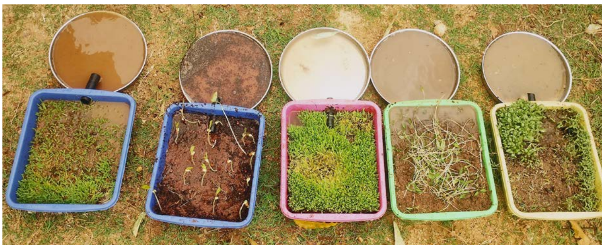
Fig. 4. Comparing soil loss. After the simulated rains, students could see for themselves that trays with more, and more diverse, plants lost less soil, while trays with fewer plants lost more soil.
